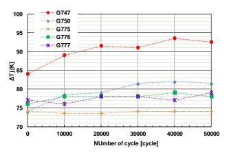
Fig.6  $\Delta$ Tj change with power cycle
