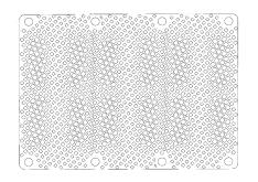
Fig.7 Example of perforated pattern of stencil
