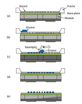
Fig.1 Work flow of grease application
