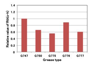
Fig.5 Thermal resistance comparison among grease types
