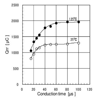
Fig. 7 Dependence of Qrr on conduction time
