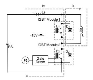
Fig.5 Current flow during transient period
