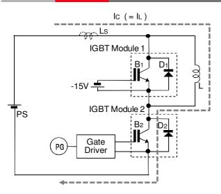
Fig.3 Current flow in ON-state of B2
