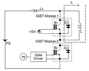
Fig.4 Current flow in OFF-state of B2
