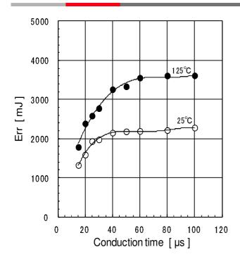
Fig. 6 Dependence of Err on conduction time
