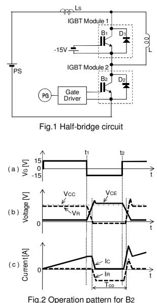
(Solid line: Waveform of B2, Dashed line Waveform of D1)
