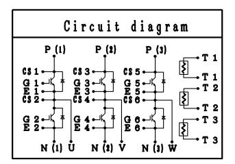
Thermistor T1, T2 and T3 are located on the same ceramic substrate with the IGBT and diode chips of phase U, V and W, respectively.
