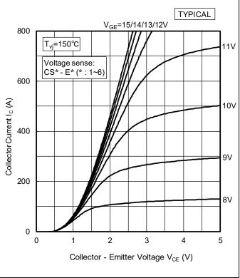
Collector Current vs. Collector - Emitter Voltage
