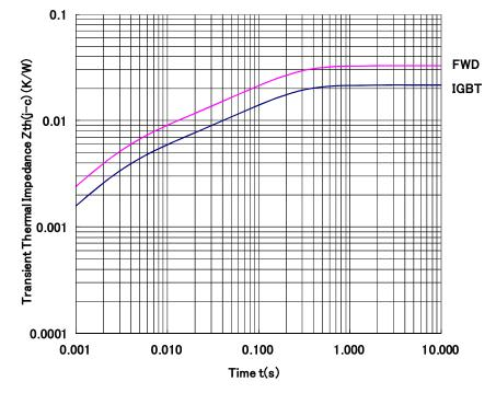
Transient Thermal Impedance Curve
