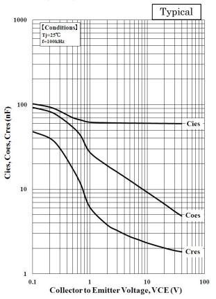
Capacitance vs. Collector to Emitter Voltage
