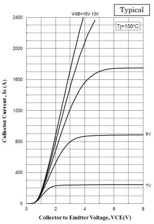
Collector Current vs.Collector to Emitter Voltage
