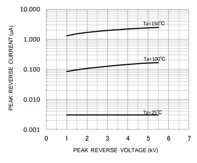
Typical Reverse Current characteristic (Ir:  $1\mu A \sim 100\mu A$ )
