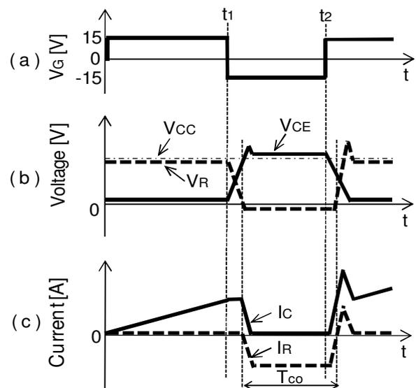
Fig.2 Operation pattern for B2
