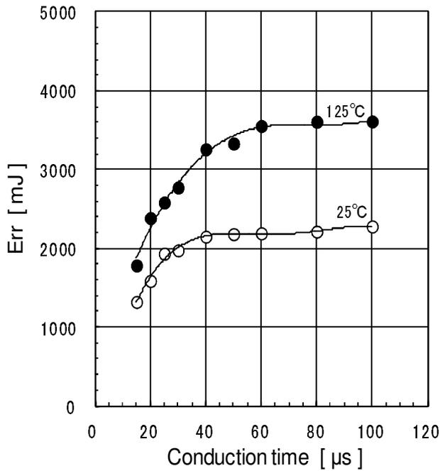
Fig. 6 Dependence of Err on conduction time
