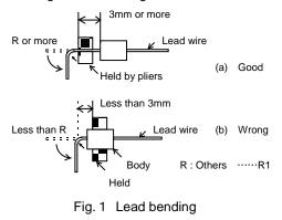
b) Bending a lead by holding its body with a pair of pliers or your fingers, as shown in Fig.1(b) must be avoided. Otherwise, the lead will be cut off or the body may get cracked. Additionally, it may result in degraded electrical capabilities and decreased reliability.
