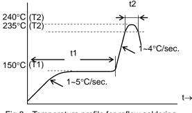
Fig.8 Temperature profile for reflow soldering (Example)
