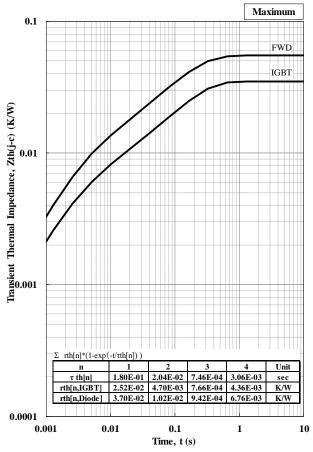
**Transient Thermal Impedance Curve**
