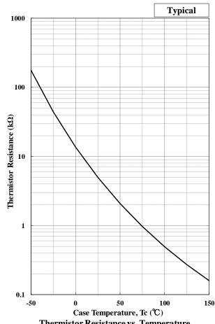
Thermistor Resistance vs. Temperature
