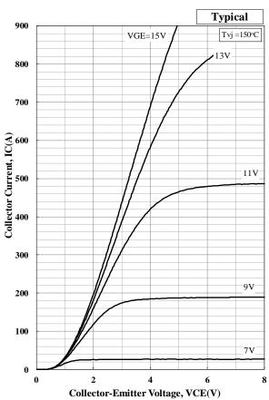
Collector Current vs. Collector to Emitter Voltage
