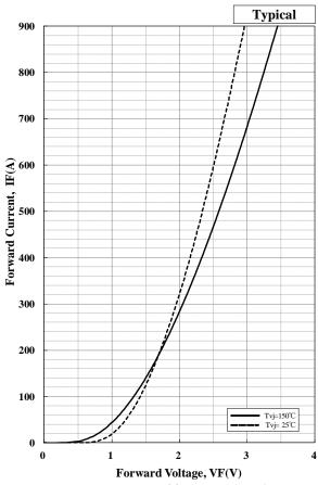
Forward Voltage of free-wheeling diode
