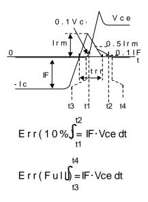
Fig.3 Definition of switching loss
