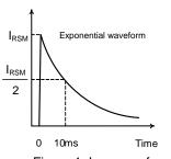
Figure 1. I<sub>RSM</sub> waveform
